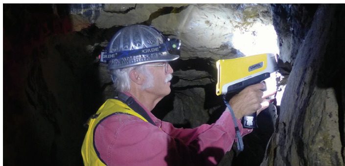
WSGS geologist uses a handheld X-ray fluorescence analyzer to check the chemistry of veins in an underground mine at South Pass City. This tool is helpful in determining the presence of critical and economic elements.
